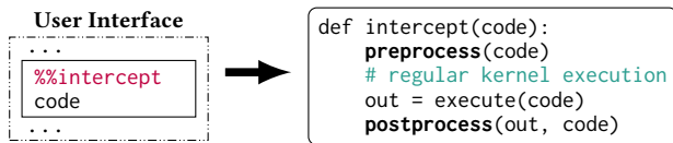
Figure 2: For every cell run, we can inject custom pre-/post-processing logic. “%%intercept” is hidden to users.
